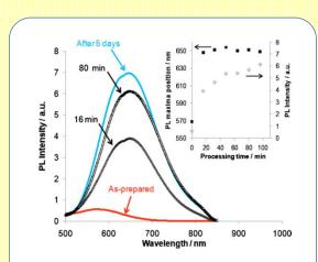
**Figure 1.** Photoluminescence (PL) spectra of Si-ncs dispersed in ethanol before and after microplasma processing at different processing time, open symbols: PL emission 5 days after processing. (*Appl. Phys. Lett.* 100, 223904, **2012**)
